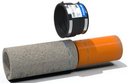
1. Mark both pipes, from the end to be connected, half the width of the coupling, less the required joint gap, which is usually 10mm.
