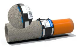
3. Align the pipes and slide the coupling onto the larger pipe, ensuring the coupling face and marked line are flush. Tighten this clamp band.
