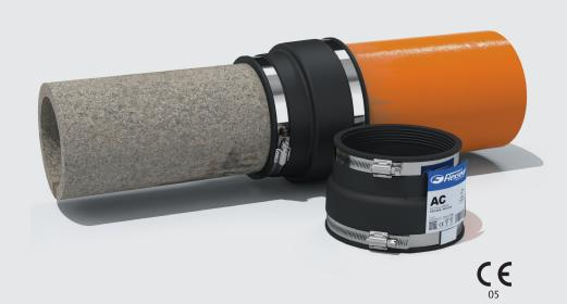
Flexseal Adaptor Couplings, sometimes referred to as reducer couplings, are designed to connect unadopted drainage pipes with different outside diameters – connecting larger drainage pipes to smaller drainage pipes and vice versa.
