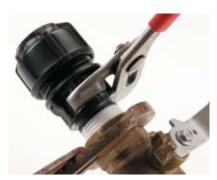
Grip the body of the 3G fitting with Multi-grips or similar plumbing tools and continue to screw the Male Adapter into the valve until tight.
